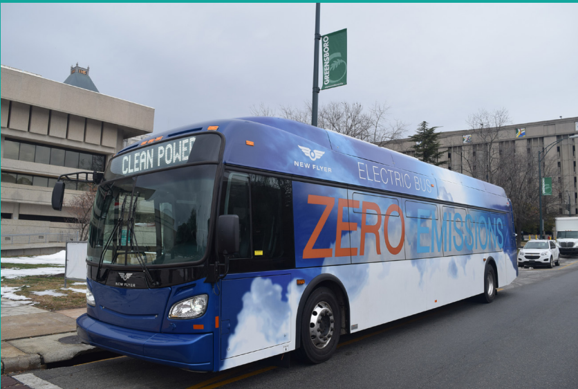
An electric bus was demonstrated in Greensboro during the recent procurement. Over the expected 12-year life cycle, each bus should save about $350,000 in maintenance versus current diesel technology, according to City officials.
