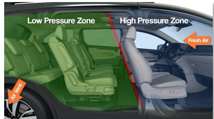
Figure 15- Illustration of Honda Odyssey modified for extra driver protection. The red line simulates a plexiglass shield, and the shaded areas illustrate HVAC concepts for added driver protection.
