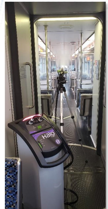
Figure 9- Disinfectant fogger on DART Light Rail Vehicle
