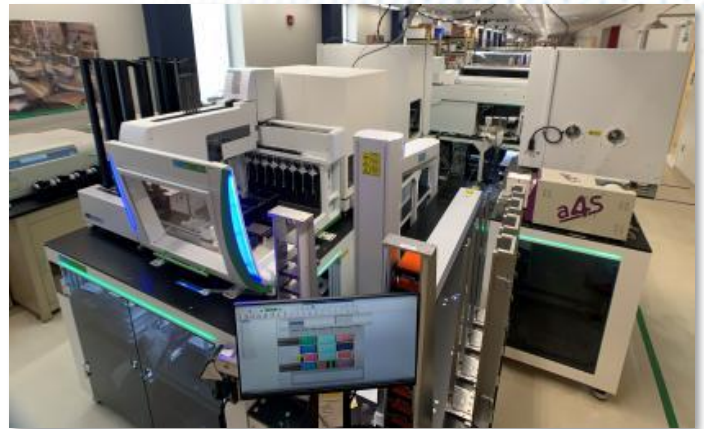
Figure 4- The automated workstation at Rutgers can process up to 10,000 SARS-CoV-2 tests per day.
