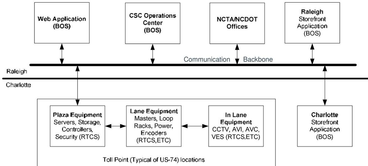
The Plaza Equipment could be located at the roadside, but since a more secure local facility (the MRTMC) exists, that is the preferred location.
