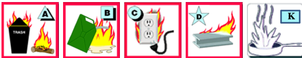
Figure 1 – pictograms used for identifying fire classes on fire extinguishers
