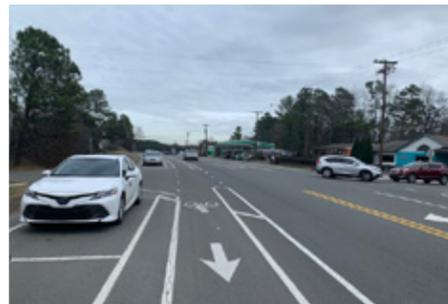
This project converted a five-lane roadway into a three-lane configuration between University Drive and Chapel Hill Road in Durham County. It added multimodal access through the addition of bicycle lanes, bus stop pull-outs, and 21 on-street parking spaces. It provided connectivity to six neighborhoods and has brought in several new local businesses along the road since the implementation of the project. This project has improved safety, reduced traffic accidents and lowered vehicle speeds.
