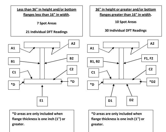
(2) Two random adhesion tests (1 test=3 dollies) per span are conducted on interior surfaces in accordance with ASTM D4541 (Adhesion Pull Test) after the prime coat has been properly cured in accordance with ASTM D4752 (MEK Rub Test) with no less than a 4 resistance rating, and will be touched up by the Contractor. The required minimum average adhesion is 400 psi.
