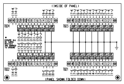
Provide permanent labels that indicate the slot and the pins connected to each terminal that may be viewed from the rear cabinet door. Label and orient terminals so that each pair of inputs is next to each other. Indicate on the labeling the input file (I or J), the slot number (1-14) and the terminal pins of the input slots (either D & E for upper or J & K for lower).
