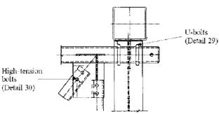
Beam-Column Connection for Truss Structure
