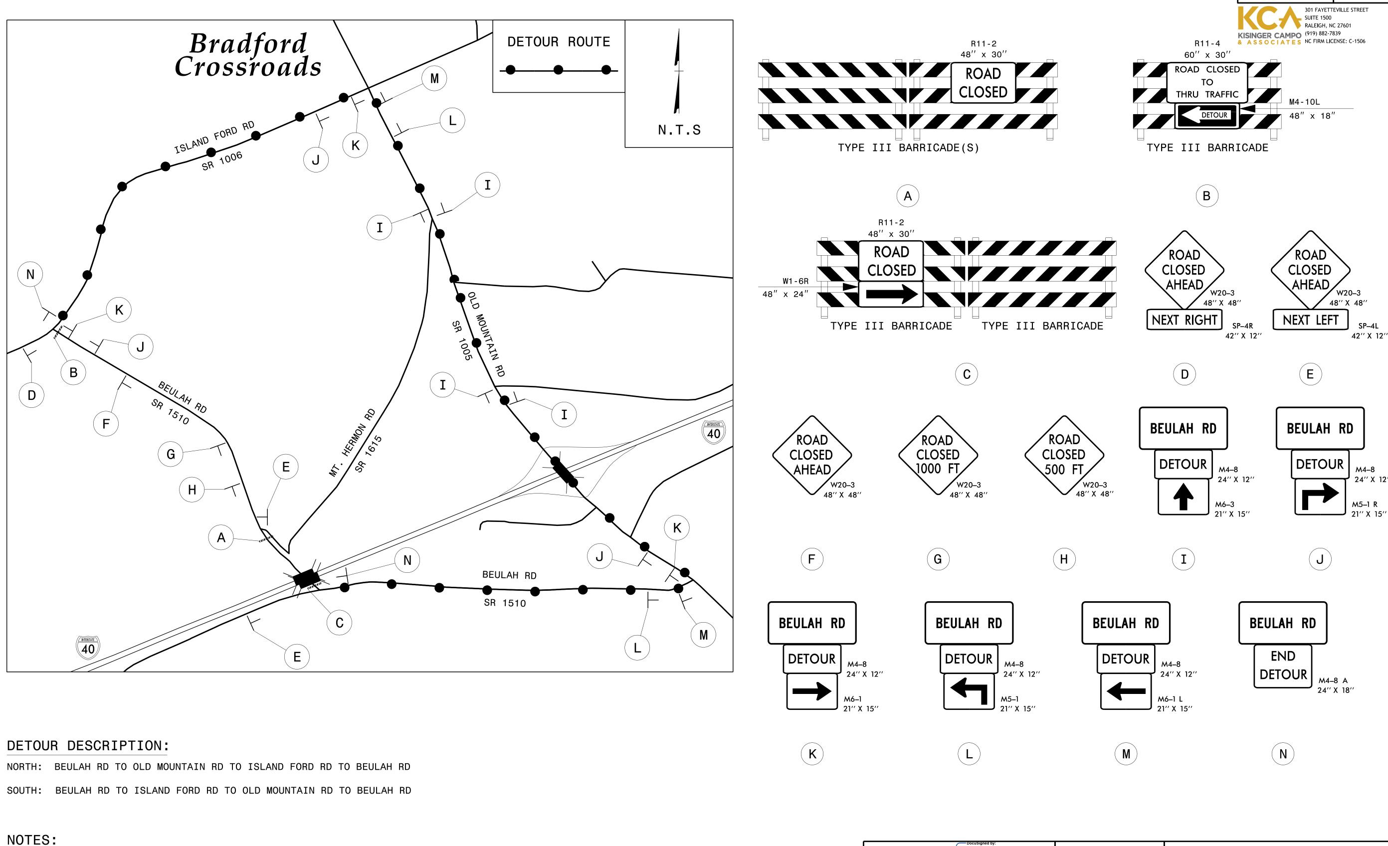
1. TRAFFIC CONTROL DEVICES (A) THRU (N) SHALL BE INSTALLED PER ENGINEER'S INSTRUCTIONS.
