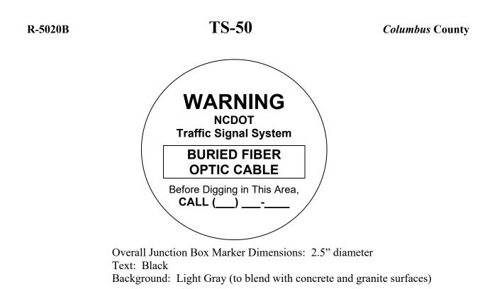
Submit samples of proposed junction marker to the Engineer for approval before installation. In lieu of designing a custom junction box marker, the Contractor may submit for the Engineer's approval a stock/standard junction box marker format (i.e., off-the-shelf format) from the junction box marker manufacturer that differs from the example format proposed above but that still embodies the content and intent conveyed by the example format.
