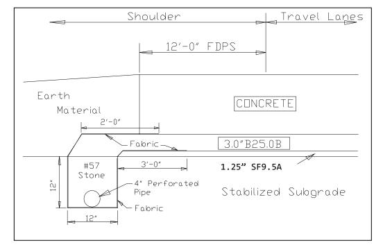
Shoulder drains are required for these projects. The detail for construction of the shoulder drains is shown above.
