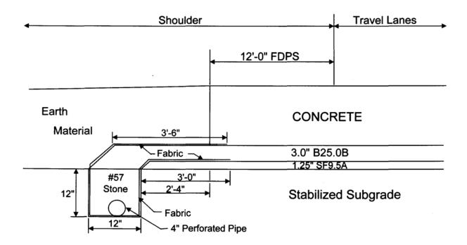
Shoulder drains are required for this project. The detail for construction of the shoulder drains is shown above.
