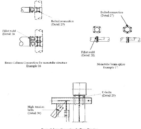
Beam-Cohunn Connection for Truss Structure Example 18
