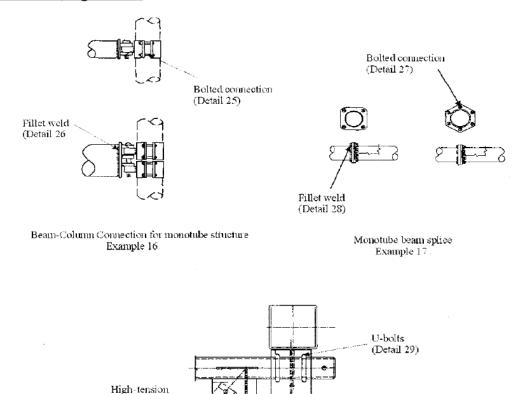
Beam-Column Connection for Truss Structure Example 18
