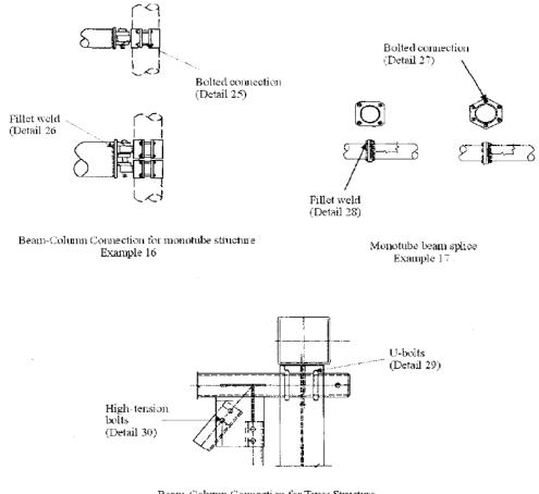
Beam-Cohumn Connection for Truss Structure Example 18
