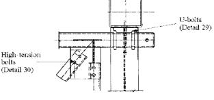
Beam-Column Connection for Truss Structure Example 18
