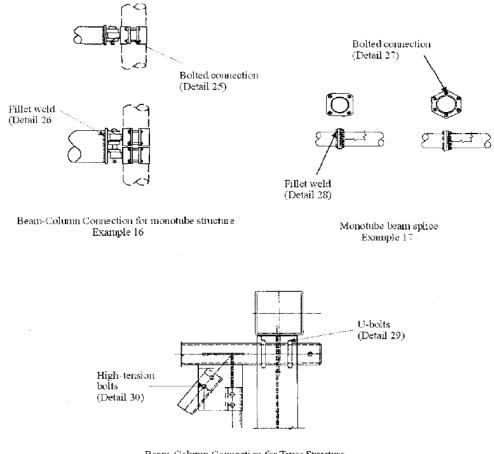
Beam-Cohumn Connection for Truss Structure Example 18
