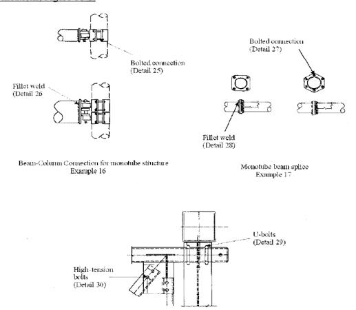
Beam-Cohumn Connection for Truss Structure Example 18
