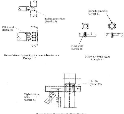
Beam-Cohunn Connection for Truss Structure Example 18
