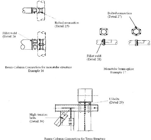
am-Column Connection for Truss Struct Example 18
