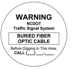
Overall Junction Box Marker Dimensions: 2.5" diameter Text: Black Background: Light Gray (to blend with concrete and granite surfaces)
