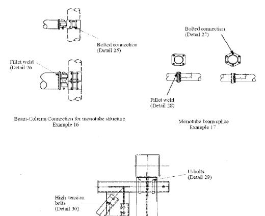
Beam-Cohmun Connection for Truss Structure Example 18
