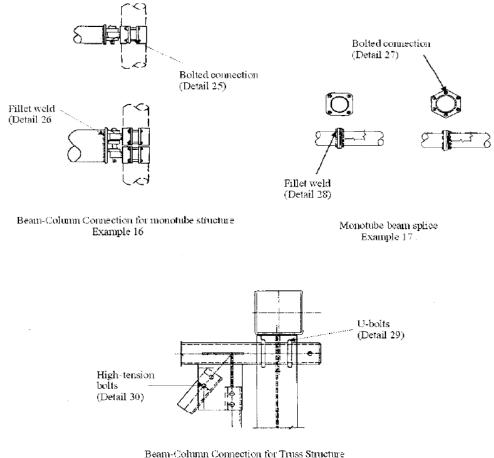
am-Column Connection for Truss Struct Example 18
