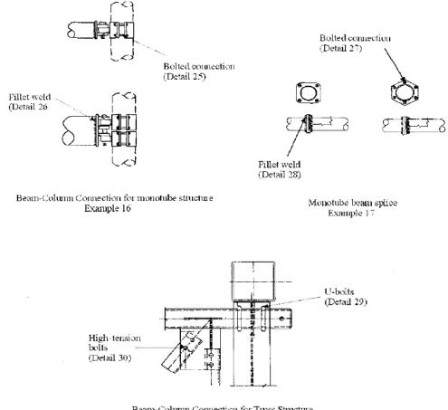
Beam-Cohunn Connection for Truss Structure Example 18
