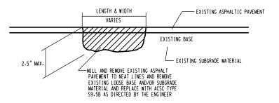
\*NOTE: EDGES OF PATCHED AREA ARE TO BE CLEANED OF ALL DEBRIS AND COATED WITH AN APPROVED TACK MATERIAL BEFORE PLACING ASPHALT.
