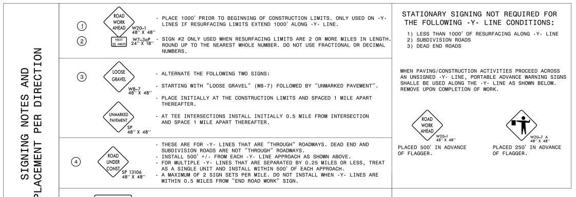
PLACE 500' FOLLOWING THE END OF CONSTRUCTION LIMITS OR AS SHOWN
