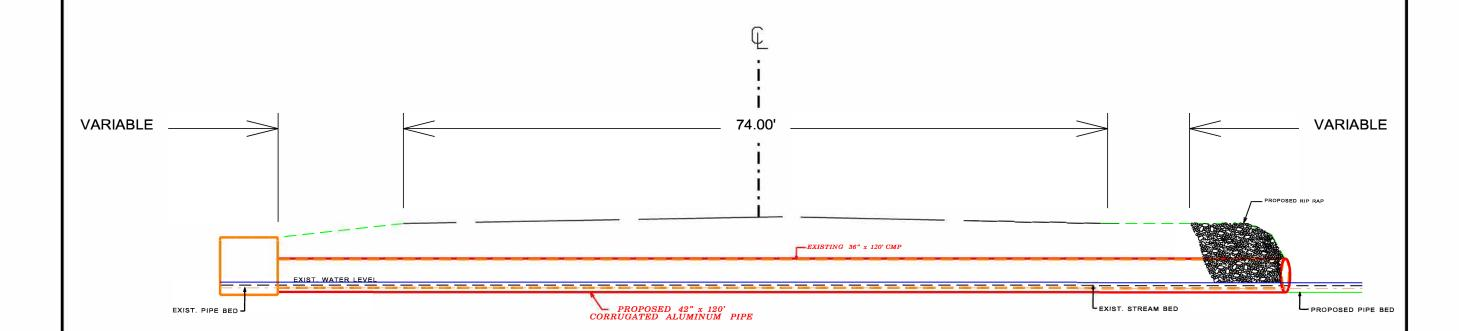
NOTES: PROPOSED 42" x 105' CORRUGATED ALUMINUM PIPE TO BE BURIED 0.7' BELOW EXISTING STREAM BED ALL ELEVATIONS BASED ON ASSUMED DATA
