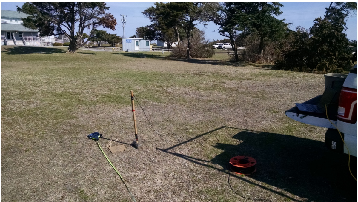
2.b. Photo showing 20-pound sledgehammer and metal plate used as energy source.
