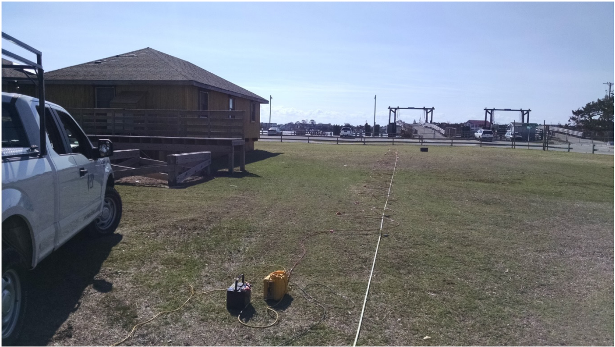
2.a. Photo looking south showing seismograph (yellow box) and geophone array laid out across site .
