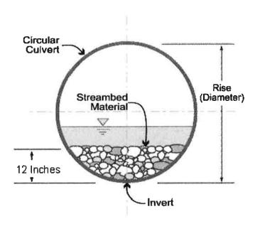
In all other areas: Culverts greater than 48 inches in diameter will be buried at least one foot below the bed of the stream. Culverts 48 inches in diameter or less shall be buried to maintain aquatic passage and to maintain passage during drought or low flow conditions, and every effort shall be made to maintain the existing channel slope.
