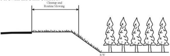
TYPICAL FILL SECTION WITH SLOPE 2:1 AND STEEPER.
