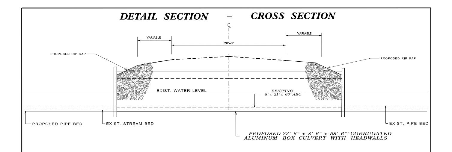
NOTES: \* PROPOSED 23'-6" X 8'-6" X 58'-6" CORRUGATED ALUMINUM BOX CULVERT TO BE BURIED 1.0' BELOW EXISTING STREAM BED
