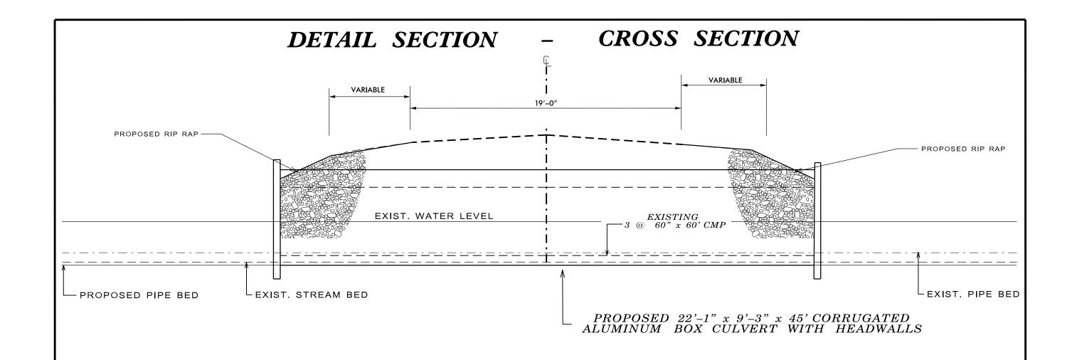
NOTES: \* PROPOSED 22'-1" X 9'-3" X 45' CORRUGATED ALUMINUM BOX CULVERT TO BE BURIED 1.0' BELOW EXISTING STREAM BED
