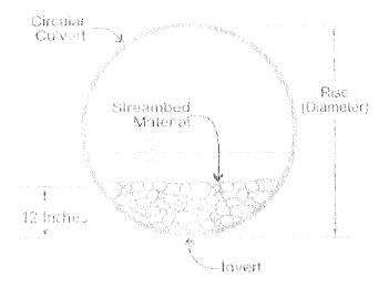
In all other counties: Culverts greater than 48 inches in diameter will be buried at least one foot below the bed of the stream. Culverts 48 inches in diameter or less shall be buried or placed on the stream bed as practicable and appropriate to maintain aquatic passage, and every effort shall be made to maintain the existing chapnel slope. The bottom of the culvert must be placed at a
