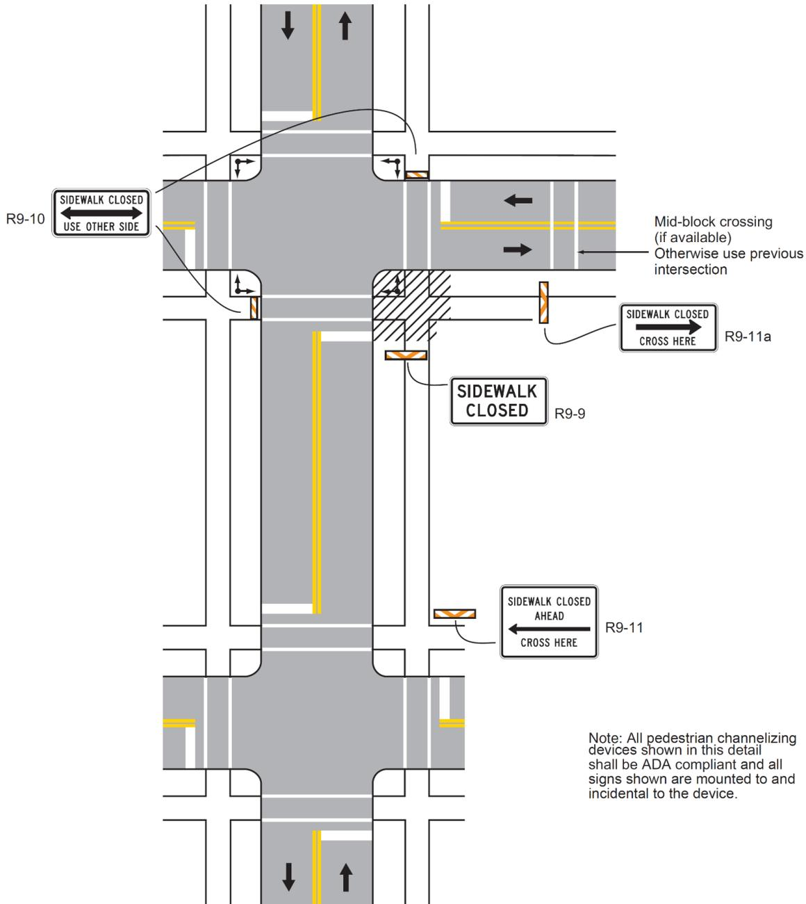
Note: All pedestrian channelizing devices shown in this detail shall be ADA compliant and all signs shown are mounted to and incidental to the device.
