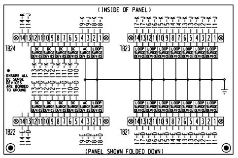
For base mounted cabinets, mount surge protection panels on the left side of the cabinet as viewed from the rear. Attach each panel to the cabinet rack assembly using bolts and make it easily removable. Mount the surge protection devices in vertical rows on each panel and connect the devices to one side of 12 position, double row terminal blocks with #8 screws. For each surge protection panel, terminate all grounds from the surge protection devices on a
