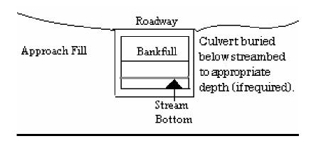
In all other counties: Culverts greater than 48 inches in diameter will be buried at least one foot below the bed of the stream. Culverts 48 inches in diameter or less shall be buried or placed on the stream bed as practicable and appropriate to maintain aquatic passage, and every effort shall be made to maintain the existing channel slope. The bottom of the culvert must be placed at a depth below the natural stream bottom to provide for passage during drought or low flow conditions.
