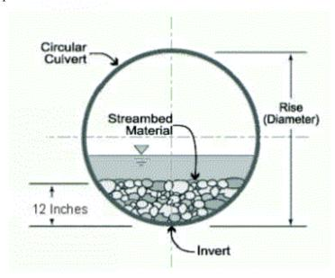
In all other counties: Culverts greater than 48 inches in diameter will be buried at least one foot below the bed of the stream. Culverts 48 inches in diameter or less shall be buried or placed on the stream bed as practicable and appropriate to maintain aquatic passage, and every effort shall be made to maintain the existing channel slope. The bottom of the culvert must be placed at a depth below the natural stream bottom to provide for passage during drought or low flow conditions.
