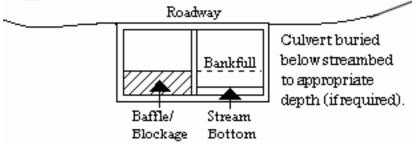
**4.1.3.** Where adjacent floodplain is available, flows exceeding bank-full should be accommodated by installing culverts at the floodplain elevation.
