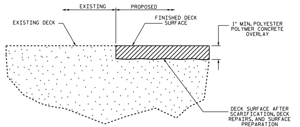
DETAIL FOR POLYESTER POLYMER CONCRETE OVERLAY
