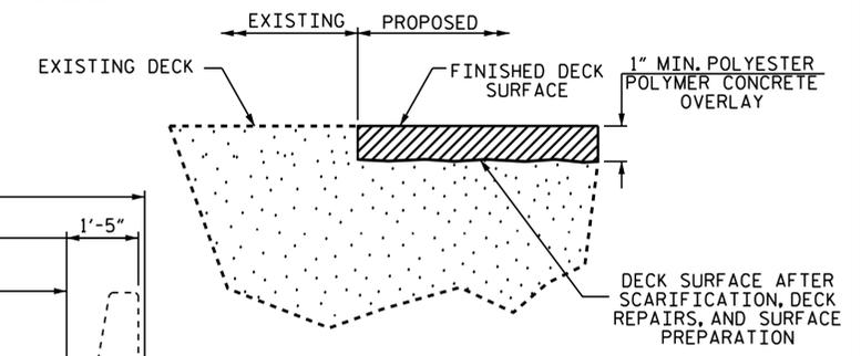
DETAIL FOR POLYESTER POLYMER CONCRETE OVERLAY
