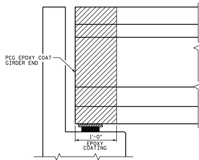
LIMITS OF PCG EPOXY COATING GIRDER ELEVATION
