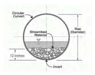
In all other areas: Culverts greater than 48 inches in diameter will be buried at least one foot below the bed of the stream. Culverts 48 inches in diameter or less shall be buried to maintain aquatic passage and to maintain passage during drought or low flow conditions, and every effort shall be made to maintain the existing channel slope.
