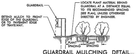
GUARDRAIL MULCHING DETAIL---USE AS DIRECTED BY FIELD ENGINEER
