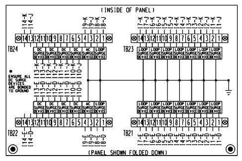
For base mounted cabinets, mount surge protection panels on the left side of the cabinet as viewed from the rear. Attach each panel to the cabinet rack assembly using bolts and make it easily removable. Mount the surge protection devices in vertical rows on each panel and connect the devices to one side of 12 position, double row terminal blocks with #8 screws. For each surge protection panel, terminate all grounds from the surge protection devices on a copper equipment
