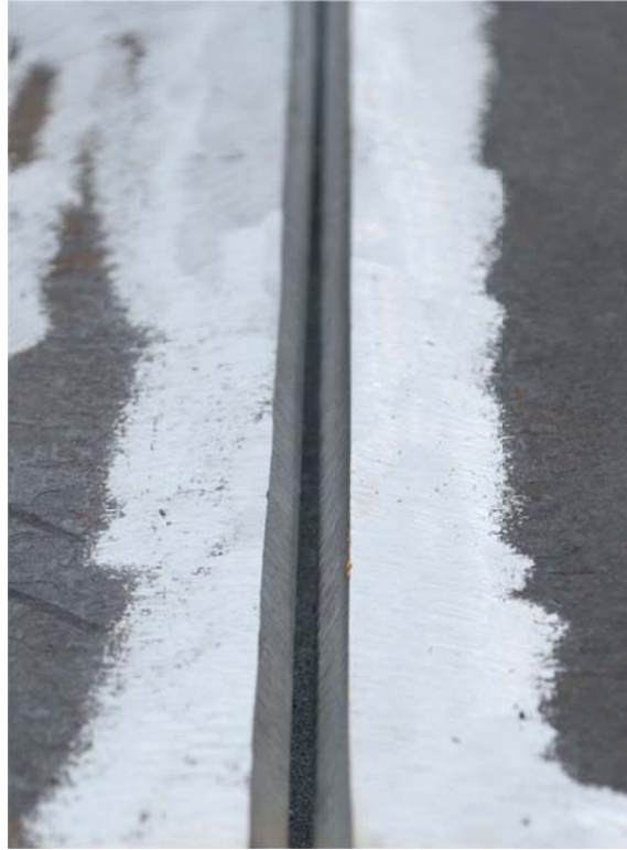
Typical fit-up using a 60 degree Single V-groove.
