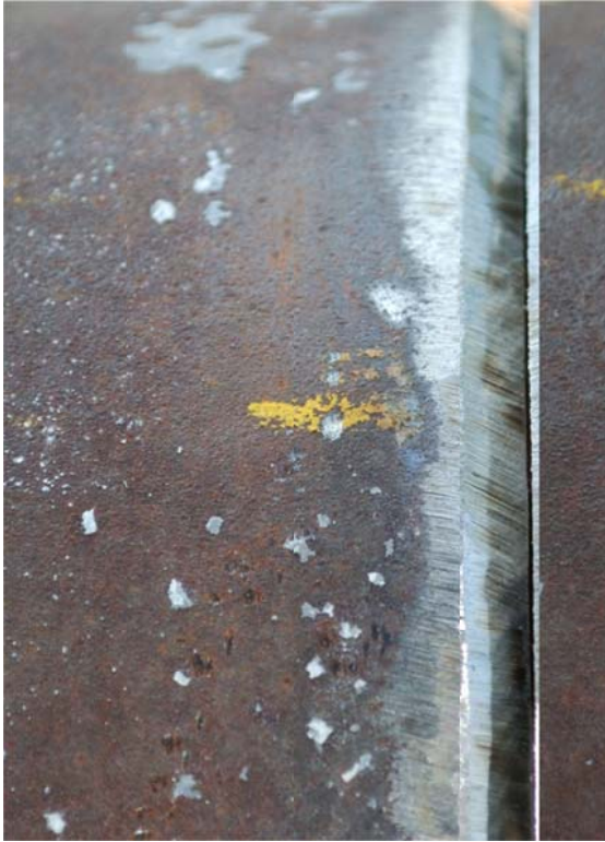
Typical fit-up using a 45 degree Single Bevel.
