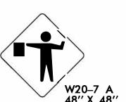
PLACED 500' IN ADVANCE OF FLAGGER. PLACED 250' IN ADVANCE OF FLAGGER.
