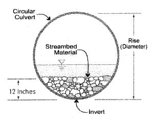
In all other counties: Culverts greater than 48 inches in diameter will be buried at least one foot below the bed of the stream. Culverts 48 inches in diameter or less shall be buried or placed on the stream bed as practicable and appropriate to maintain aquatic passage, and every effort shall be made to maintain the existing channel slope. The bottom of the culvert must be placed at a
