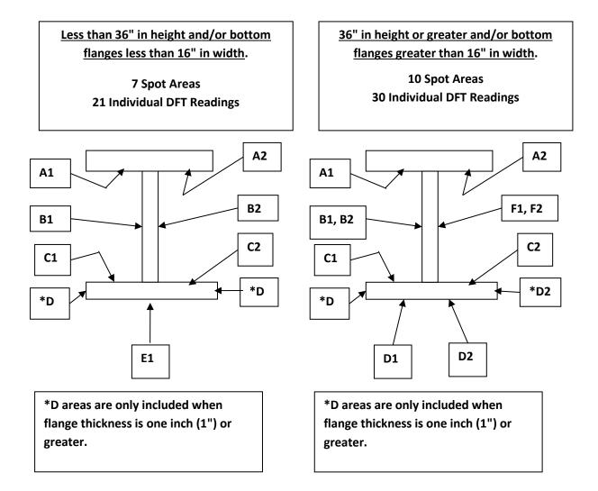
Two random adhesion tests (1 test=3 dollies) per span are conducted on interior surfaces in accordance with ASTM D4541 (Adhesion Pull Test) after the prime coat has been properly cured in accordance with ASTM D3363 (Pencil Hardness) with no less than 2H, and will be touched up by the Contractor. The required minimum average adhesion is 400 psi.
