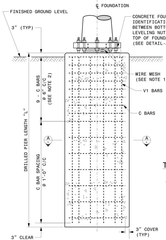
CONCRETE SHAFT ELEVATION
