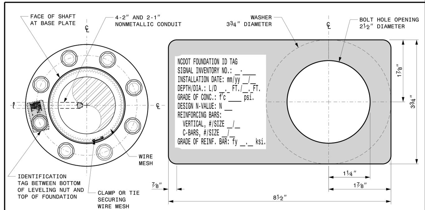
CONCRETE FOUNDATION IDENTIFICATION TAG DETAILS
