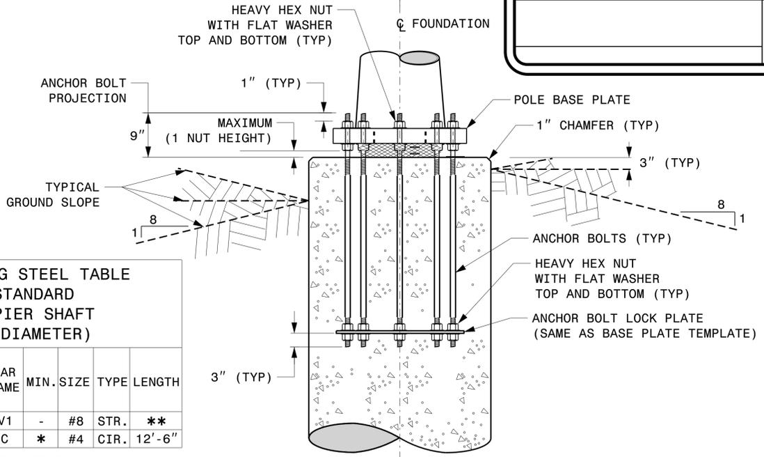
TYPICAL FOUNDATION ANCHOR BOLT DETAILS
