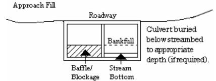
**4.5.3.** Where adjacent floodplain is available, flows exceeding bank-full should be accommodated by installing culverts at the floodplain elevation.
