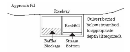
**3.6.3** Where adjacent floodplain is available, flows exceeding bank-full should be accommodated by installing culverts at the floodplain elevation. Additional culverts or culvert barrels at such crossings should not be buried, or if buried, must have sills at the inlets to ensure that they only receive flows exceeding bank-full.
