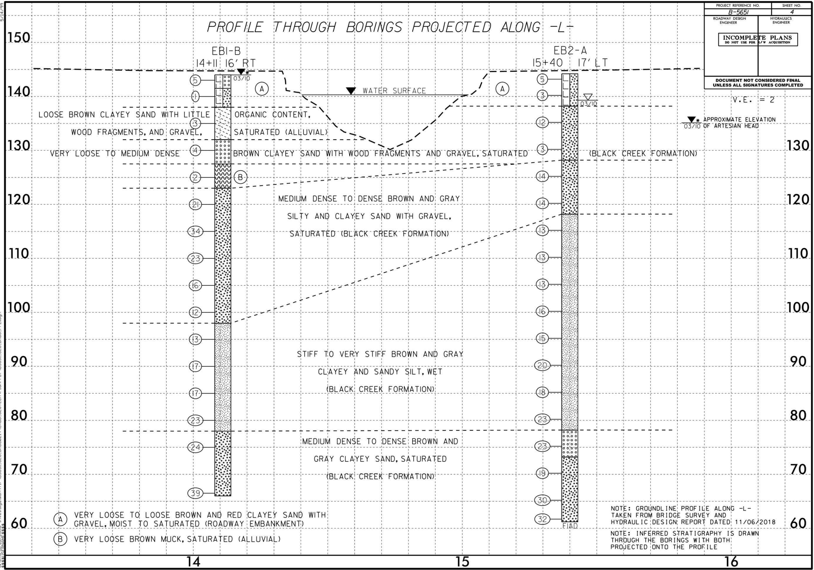
LOOSE BROWN CLAYEY SAND WITH LITTLE WOOD FRAGMENTS, AND GRAVEL, SATURATED (ALLUVIAL)
