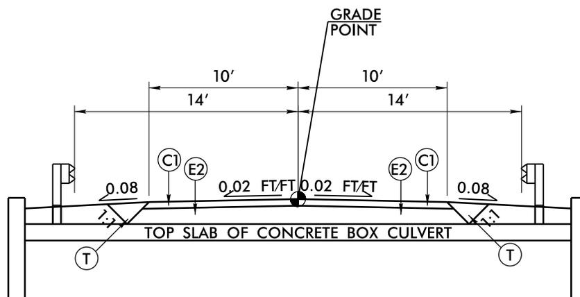
USE TYPICAL SECTION NO. 2 IN LOW FILL CONDITIONS AS DIRECTED BY THE ENGINEER
